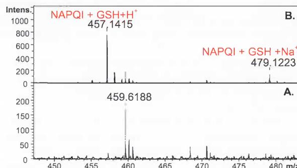
Fig. 8. Zoom in of mass range from  $m/z$  of 447 to 483. (A.) ReactorCell OFF, (B.) Reactor Cell  $E_c=800mV$ . Peak at  $m/z$  of 457.1415 corresponds to protonated ion of conjugation product. The peak of  $m/z$  of 479.1223 was identified as its  $Na^+$  adduct.
